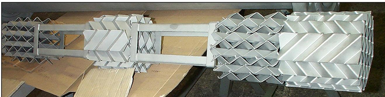
**Figure #7:** The incorporation of spacers between GV mixing elements improves the degree of mixing achieved by taking advantage of the strong turbulent eddies created at the outlet of each mixing element.
