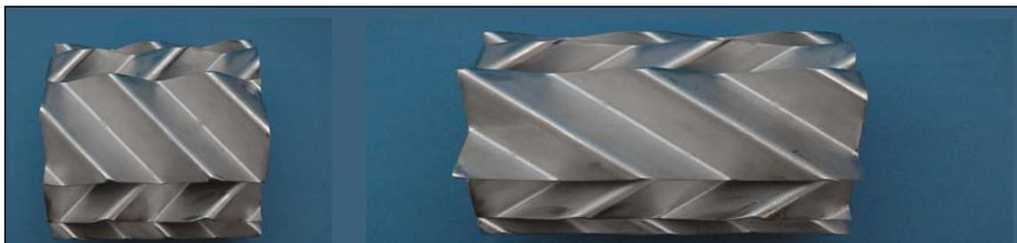
**Figure #6:** The GV mixing element pressure drop can be dramatically reduced by simply changing the corrugated plate angle relative to the pipe axis. Shown at left is the standard GV mixing element ( $L/D=1.0$ ) with a  $45^\circ$  corrugation angle relative to the pipe axis. At right is the lower pressure drop GV-L mixing element ( $L/D=1.73$ ) with a  $30^\circ$  corrugation angle.
