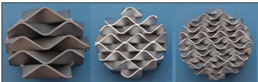
**Figure #5:** The GV mixing element is unique in its ability to “dial-in” the degree of mixing achieved by simply changing the number of mixing layers (corrugated plates) in a specific pipe size. The greater the number of mixing layers (corrugated plates) in a specific diameter, the higher the degree of mixing achieved in a fixed length. The example above shows, from left-to-right, 5 layer, 8 layer and 12 layer mixing elements that fit into the same pipe diameter.
