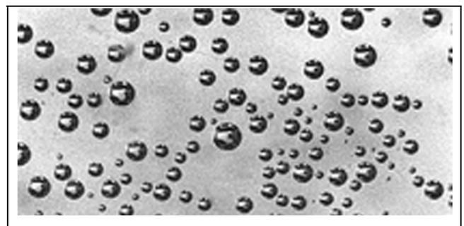
**Figure #4:** The even shear field generated by the GV mixing element assembly creates droplets of consistent size in air-water and immiscible liquid systems and distributes them evenly over the entire pipe cross-section.
