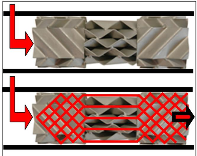
**Figure #3:** Flow pattern through three (3) GV mixing elements of 5 layer construction. Note that adjacent mixing elements are oriented 90° relative to each other.
